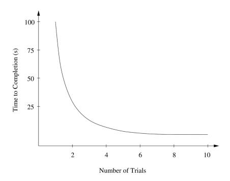
This type of curve is called a power law, because performance varies as time raised to some negative power. For example, in the figure above, time to completion is proportional to the number of trials raised to minus two (or equivalently, one over the number of trials squared). Pretty much every human skill follows a power law, with different powers for different skills. (In contrast, Windows never gets faster with practice—something for Microsoft to work on.)
