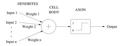
The higher an input's weight, the stronger the corresponding synapse. The cell body adds up all the weighted inputs, and the axon applies a step function to the result. The axon's box in the diagram shows the graph of a step function: 0 for low values of the input, abruptly changing to 1 when the input reaches the threshold.
