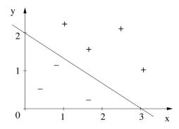
This is because the boundary is the set of points where the weighted sum exactly equals the threshold, and a weighted sum is a linear function. For example, if the weights are 2 for x and 3 for y and the threshold is 6, the boundary is defined by the equation 2x + 3y = 6. The point x = 0, y = 2 is on the boundary, and to stay on it we have to take three steps across for every two steps down, so that the gain in x makes up for the loss in y. The resulting points form a straight line.
