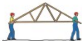
Two operatives carrying truss
