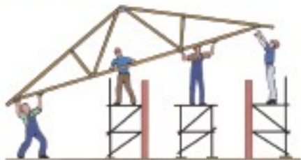
Lifting truss into position using manhandling method
