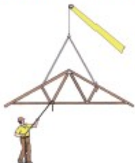
Lifting truss into position using a crane and a guide rope
