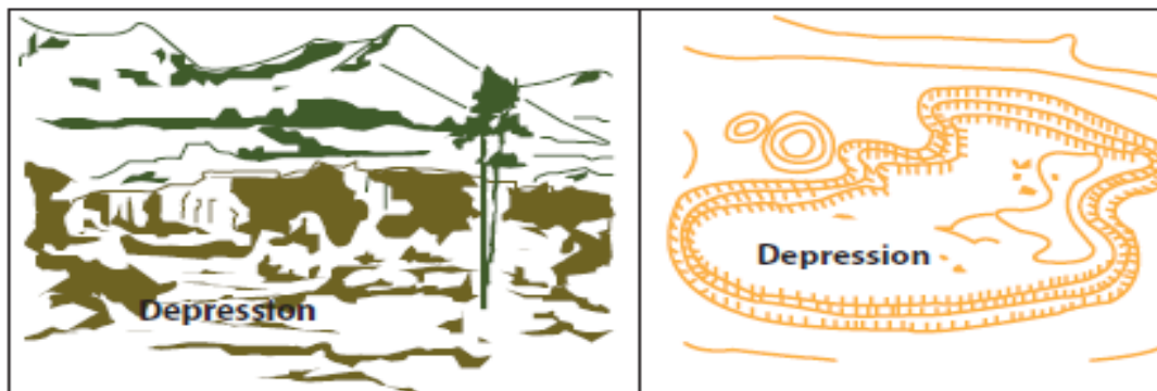
Figure 2.31: A depression and its representation on a contour map
