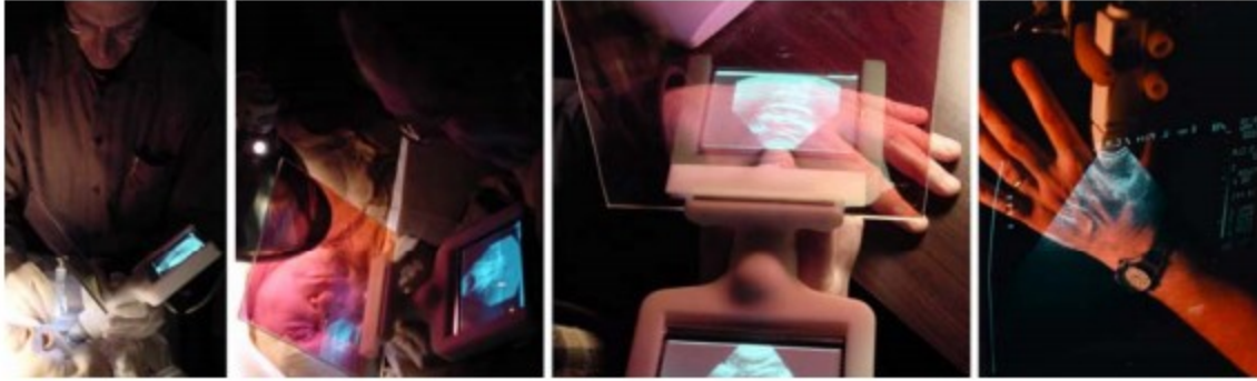
F. The Sonic Flashlight uses a see-through display to overlay real-time ultrasound images over a patient's body parts[20]
