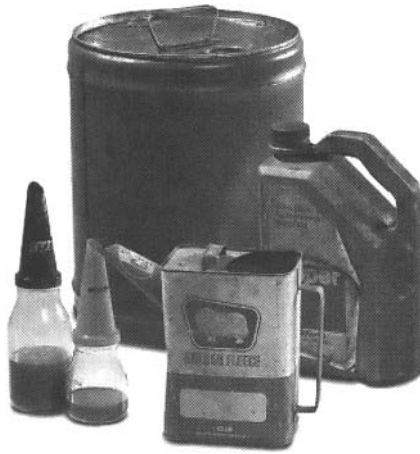
Figure 12.2: Unsuitable lube transfer containers.
