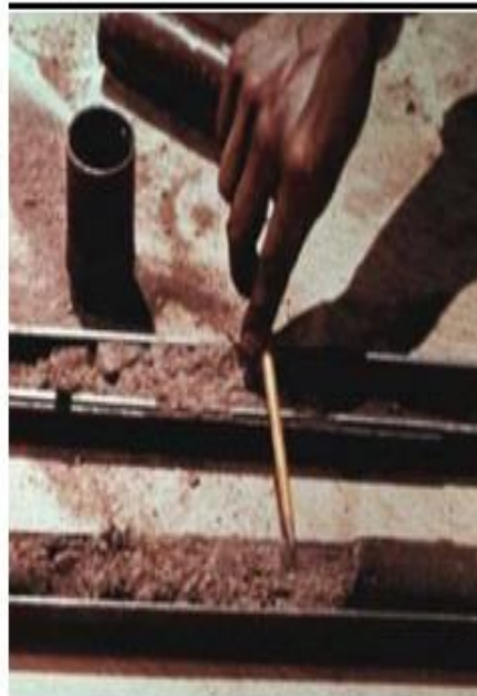
Open sampler with soil sample and cutting shoe
