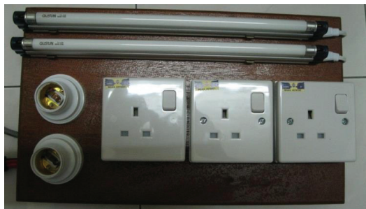
Figure 21: Appliance Board Top View. The board features two 8W fluorescent, two 20W light bulbs and three three-pin switches
