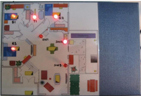
Figure 24: LED Output from PIC on Map. Referring to previous figure, the corresponding outputs are switched ON
