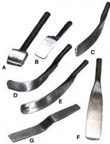
A)spoon dolly B)light dinging spoon C)surfacing spoon D)Inside high crown E)Inside medium crown F)inside heavy-duty spoon G)bumping file
