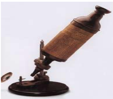
Figure 4.3 Robert Hooke's microscope
