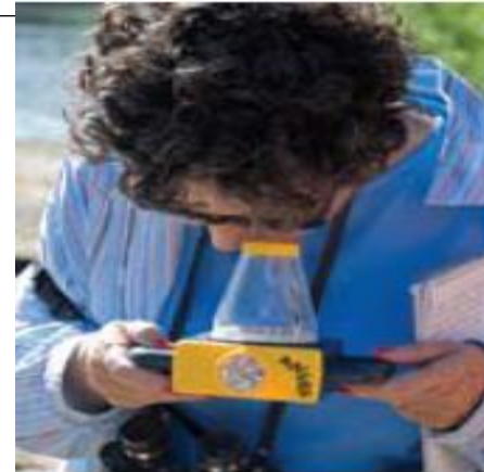
Figure 1.26 A field microscope – this is used to investigate the structure of specimens in the field, whilst still fresh
