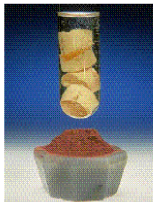
Figure 3.3 White and red phosphorus are two allotropic forms of the element. White phosphorus consists of P_4 molecules; red phosphorus involves P_4 units bonded to one another in a chain. (C. D. Wiley)
