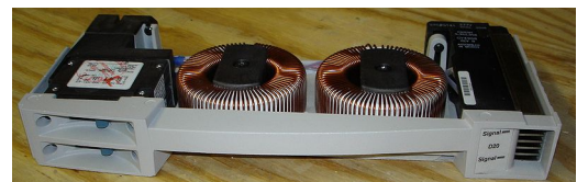
A pair of modern 2.4 kW dimmers by Electronic Theatre Controls
