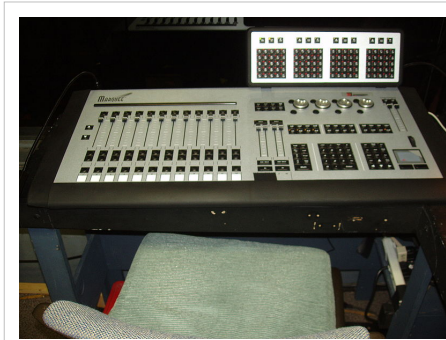
Entertainment Technology's Marquee lighting console.
