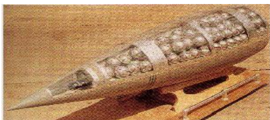
Fig. 2-53. A chemical warhead for the Honest John rocket. It was designed to break apart and disperse the spherical bomblets of nerve agent. Photograph: Chemical and Biological Defense Command Historical Research and Response Team, Aberdeen Proving Ground, Md.
