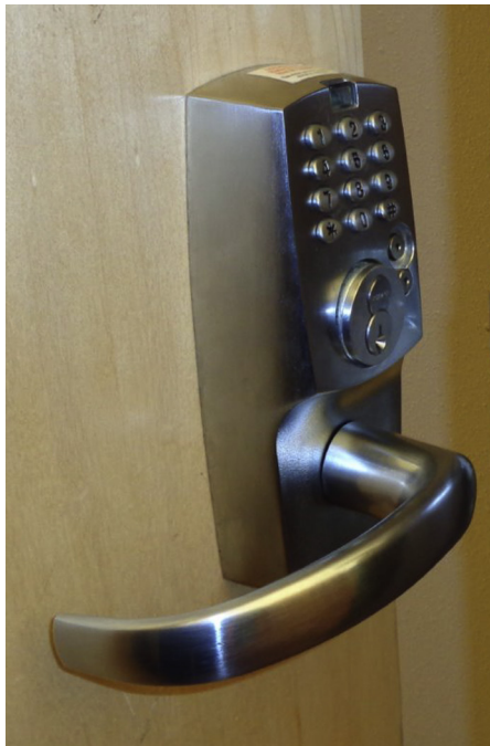
FIGURE 12.1 Example of one of the many cipher locks being used in businesses.
