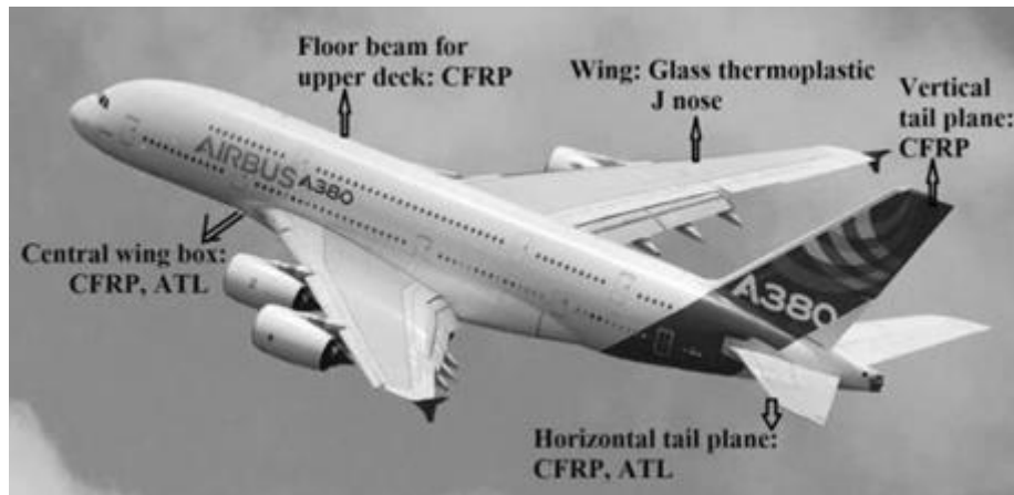
Figure 1: Composite Materials used in Airbus 380 [9].
