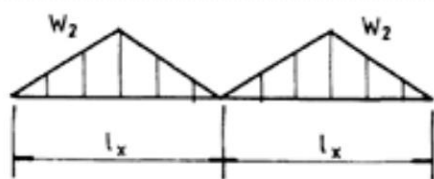
Floor load on beam BB
