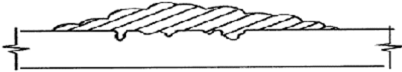
Figure 20-7 Illustration of Pits Forming Beneath Bacterial Deposit
