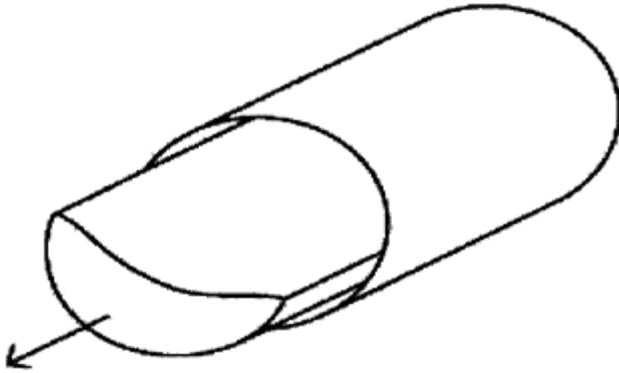
Figure 23-14 Insertion Liner Pulled Into Pipe
