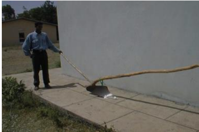
Figure 4: The maresha modified plow
