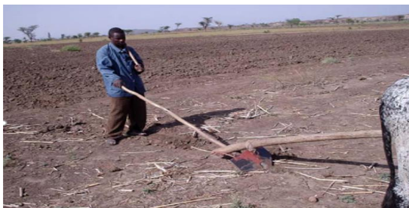
Figure 2: the maresha modified tie-ridger
