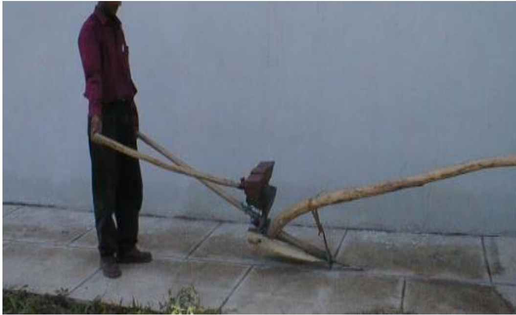
Figure 5:the semi automatic row planter.
