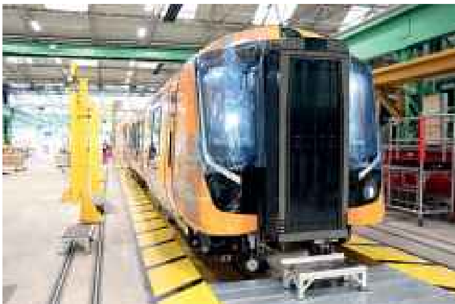
First '730': the first of 36x3-car sets for the Cross City line in Birmingham under construction in 'G' shop at Litchurch Lane; Bombardier will also build 45x5-car '730s' for West Midlands Trains' London Northwestern Railway services. Philip Sherratt
