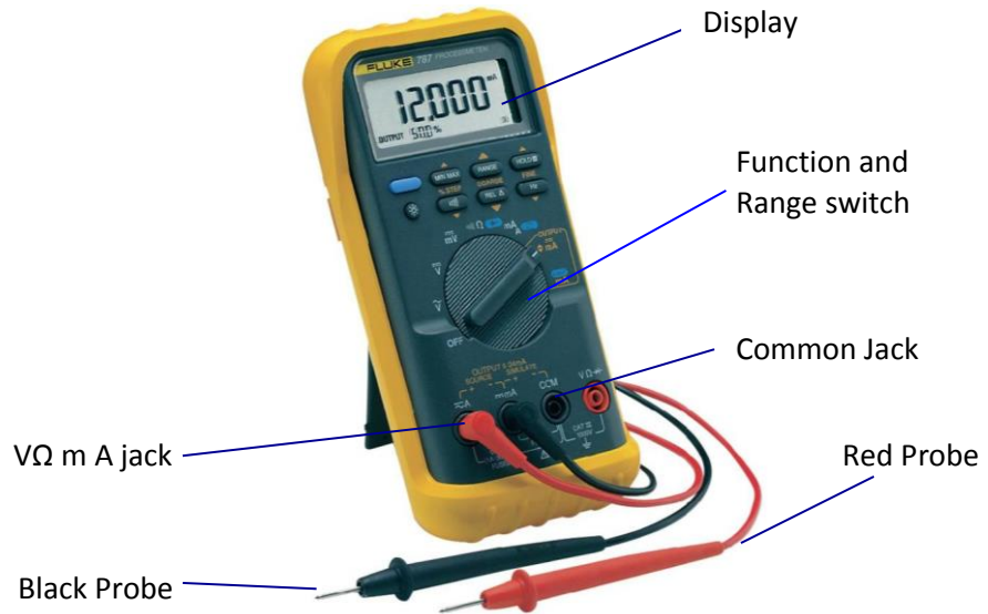
Figure 29: Parts of a multimeter
