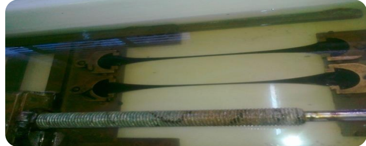
Fig : 12. Ductility of Asphalt Mold and testing machine while in test
