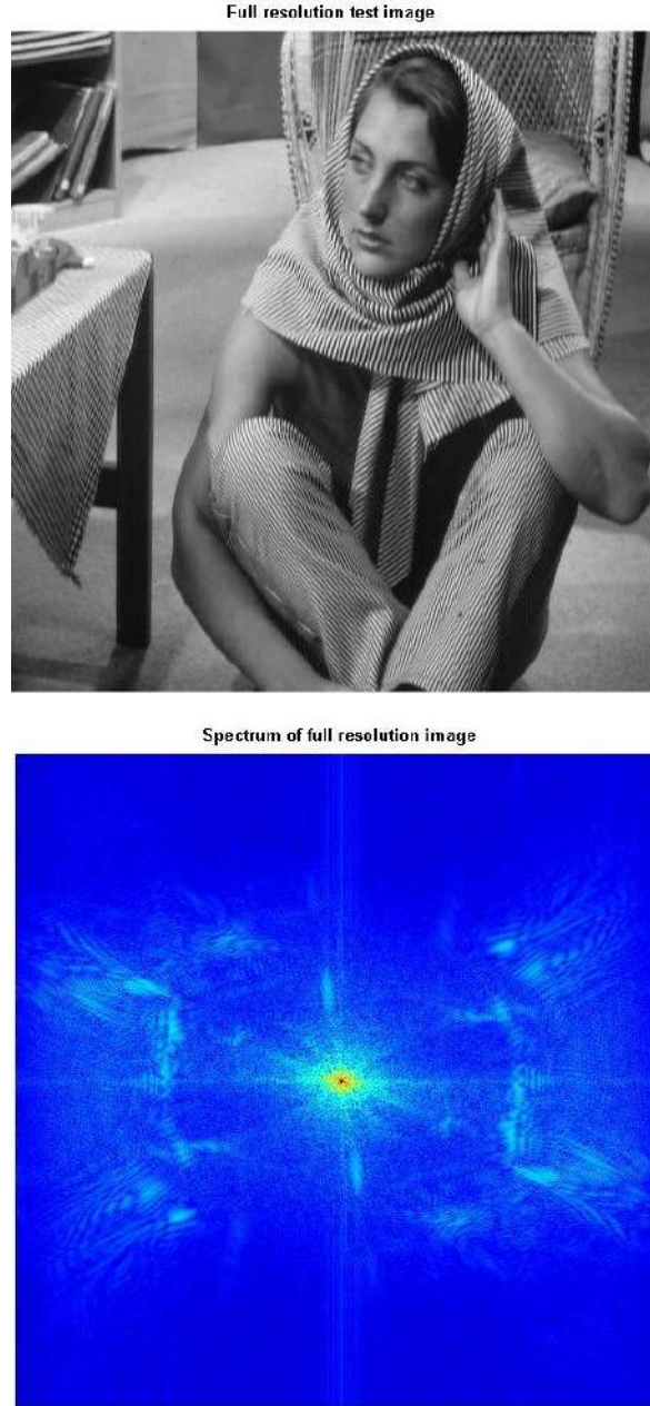
Fig. (3.4). A full resolution test image (upper) and module of its Fourier spectrum centered at zero spatial frequencies (f_x, f_y) and displayed in false colors (MATLAB ® color map "jet") for better visibility of its high-frequency components (bottom).
