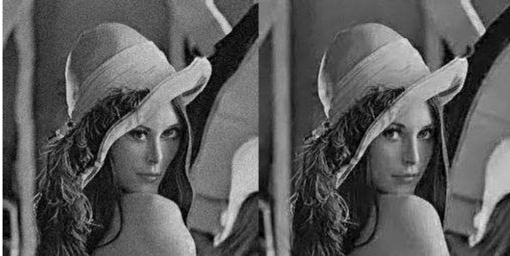
Fig. (9.19). An example of image resampling from irregular to regular sampling lattice and denoising in sliding window: noisy and irregularly sampled image (left) and resampled (rectified) and denoised image (right).
