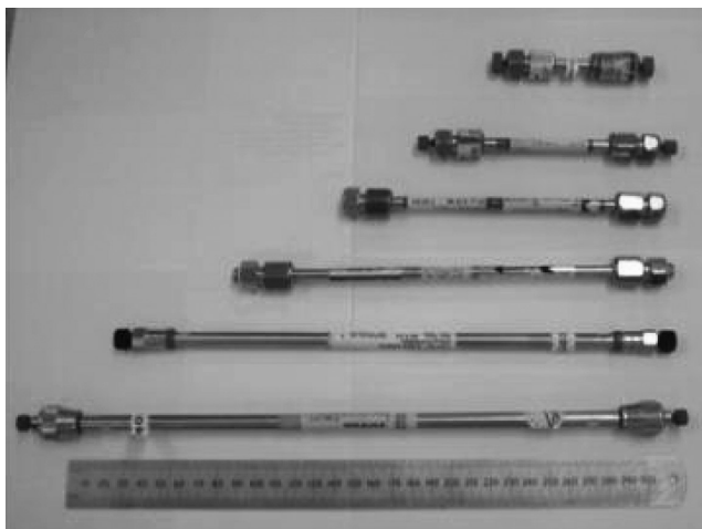
Figure 1.2 Different lengths of a chromatography column.
