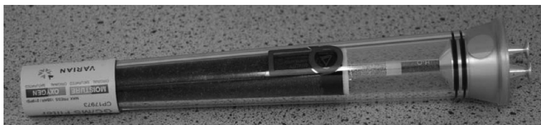
Figure 2.3 An example of an in-line trap to remove moisture and oxygen.
