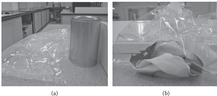
Figure 8.29 (a) Packaging used to sample fire debris at a scene; (b) example of fire debris sealed in a nylon bag.
