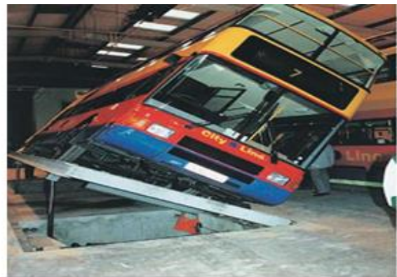
Figure 5.25b A double-decker bus being tilted to test its stability
