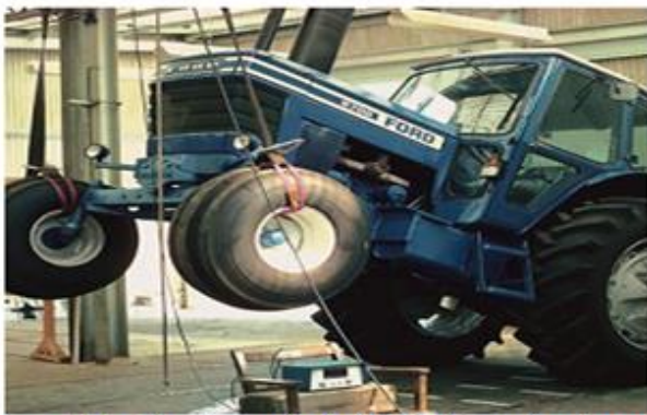
Figure 5.25a A tractor under test to find its center of gravity
