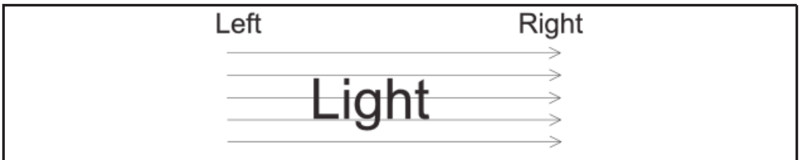
Figure 3-3. It is the convention in light ray diagrams that light is always drawn traveling from left to right.
