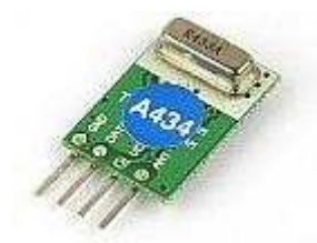
Figure 2.12. RF Based Wireless Remote Control System receiver module [21]
