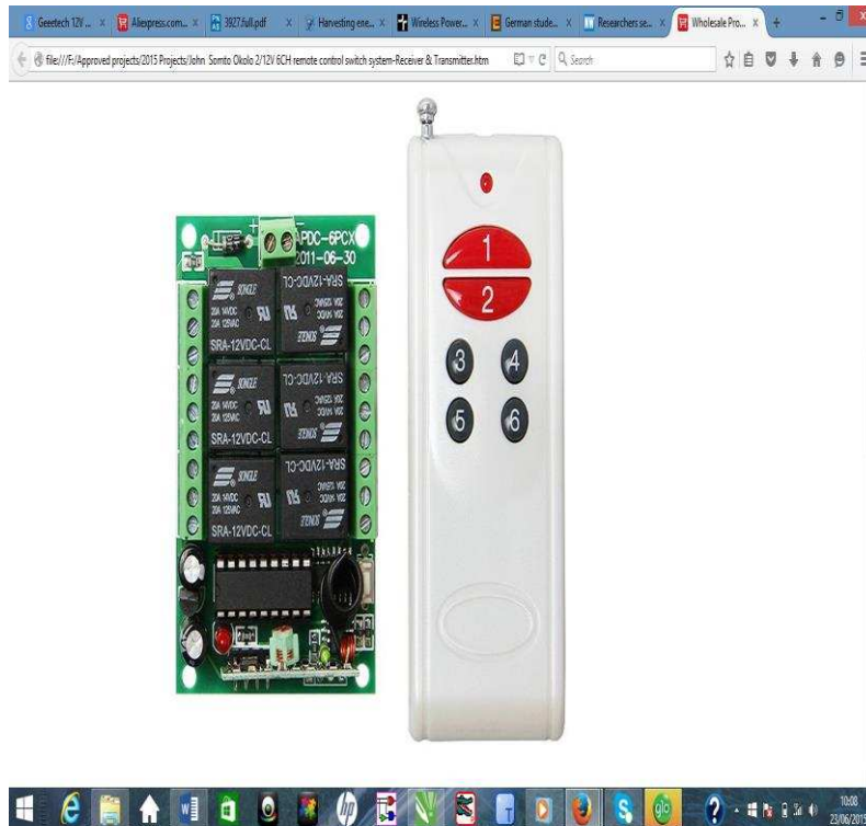
Figure 3.5. Picture of the front view of the 6 channel RF Wireless smart receiver controller
