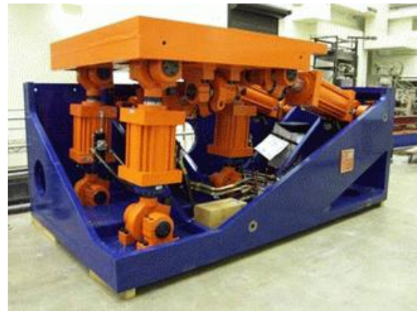
Figure 5-2: LBCB resting on lab floor.
