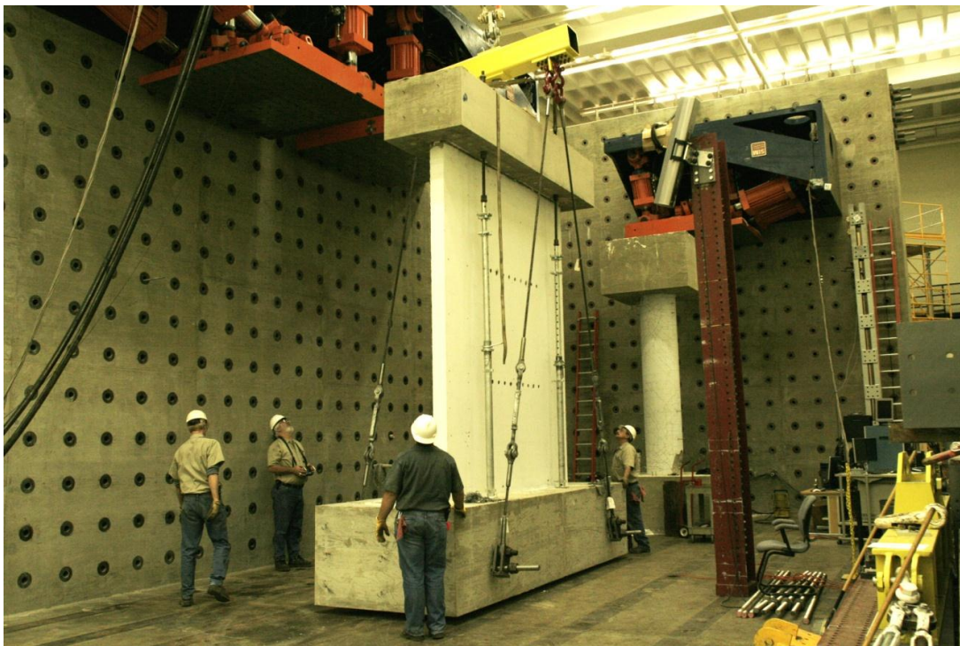
Figure 4-3: Moving a planar test specimen into the testing location (similar for CW1).
