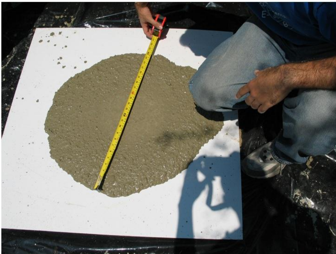
Figure 3-2: Self-consolidating concrete inverted cone test.
