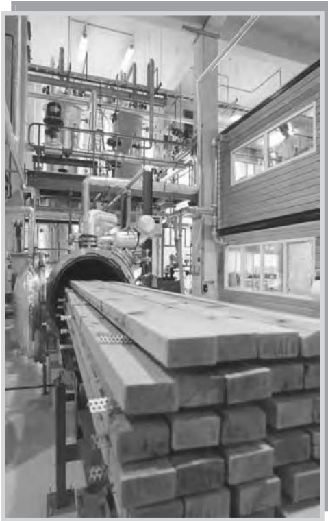
4.11 Wood leaving an acetylating tank, AKBV plant, Arnhem, the Netherlands, 1998.
